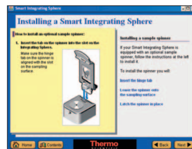
Tutorial illustrating the installation of the optional sample spinner
